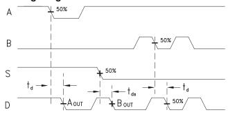
td = propagation delay, A or B to Dout tds = propagation delay, Select to Dout
